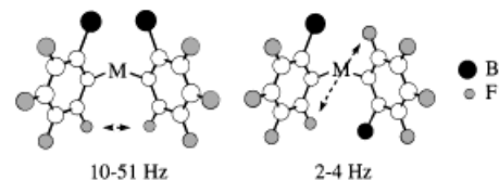
Figure 1. F-F coupling constants measured in [Pd(2\text{-}C_6BrF_4)_2L_2] complexes
